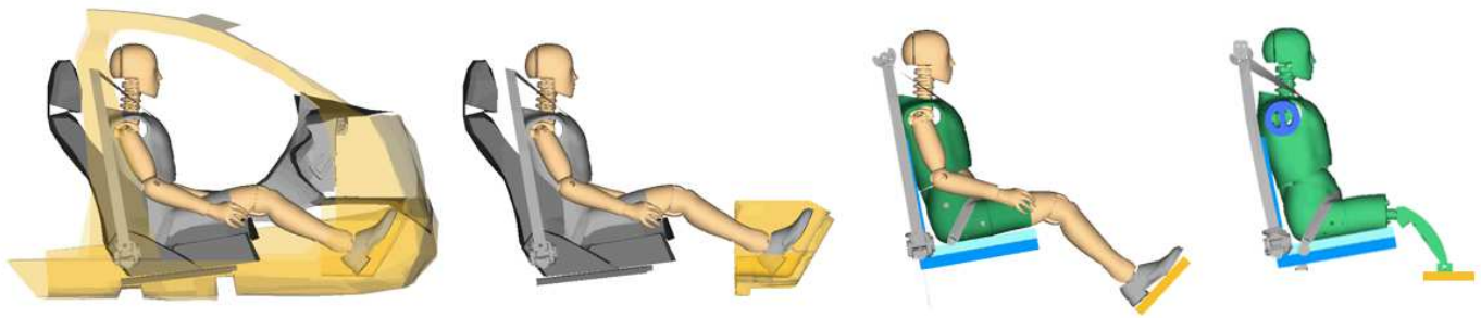
Figure 14 (A) Validated full safety system (FSS) from a midsize sedan (PGV) with (left picture, result in Figure 15: black continuous line) and (B) without airbag system (center left picture, result: black dashed line) is transferred to a configuration with identical anchor point geometry, same H350 (H-angle) (C) but seated on a steel seat with a seating surface tilted by 10° and fixed foot rest position as in FSS (center right picture, result: green dotted line). (D) Simplified bench test setup called “Torso at seat” (T@S) with under legs replaced by a hinged stiff gear and a viscous 1 kN damper, H350 arms substituted by lumped masses of 3 kg fitted to the shoulder hinges (right picture, result: green continuous line).
