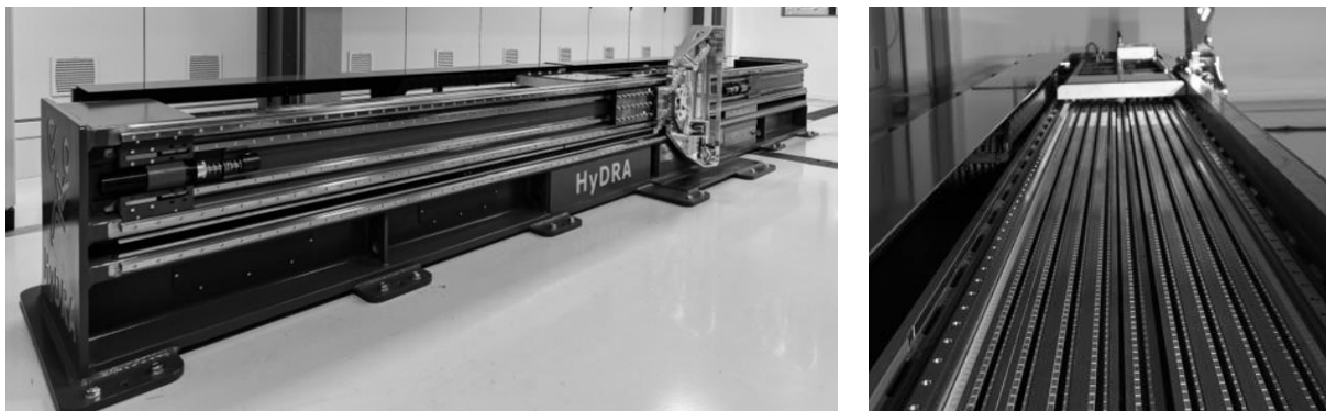
Figure 1 Nine electric linear motors mounted under a carbon-fiber sled and emerged into 6 m long magnet tracks (right-hand picture) powering closed-loop controlled HyDRA ® test bench.
