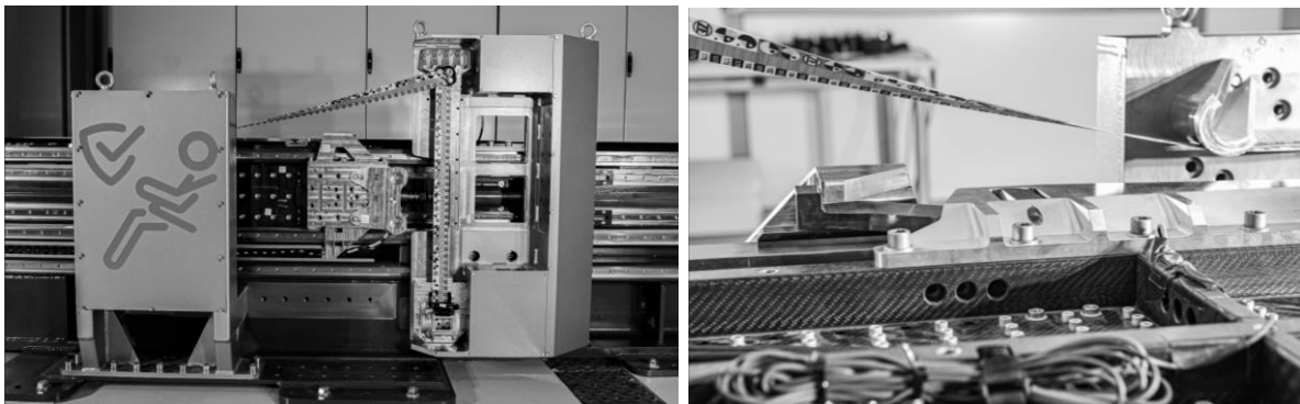
Figure 4 Linear guided mass, coupled to the sled, is first accelerated to a defined speed and then either be decoupled to impact as a free-floating mass on the seatbelt system (see decoupling mechanism on right picture) or stay coupled to be driven displacement controlled into it to load the SBS. The Seatbelt is strapped into two stiff static frames, mounted at the base of the bench. Seatbelt retractors, with engaged locking mechanism, can be mounted in various mounting positions via adaptors to the first base.
