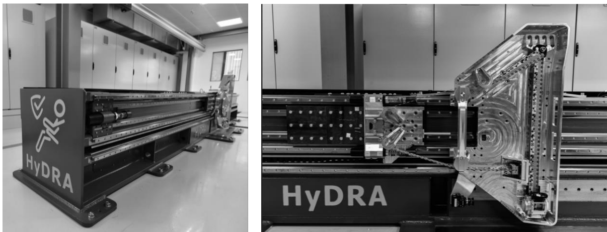
Figure 5 Front seat frame (right hand) coupled to the sled and guided in ball bearings along the three outer rails visible aside of the bench. A free-floating mass is guided along the two inner tracks, which are set back into the base such that two dampers, fixed to the base, hit the mass in its center to stop it. Beyond the central damper is a safe harbor for the frame, which cannot be reached by the free-floating mass. Alternatively, the frames may also be used to stop the free-floating mass, which is equipped with two additional dampers. An onboard high-speed camera is mounted on the frame to monitor the retractor behaviour.
